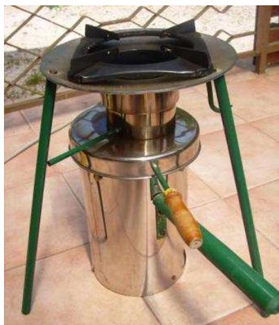
The small TLUD (top lit up draft) stove is suitable for household biochar production and is used in developing countries for cooking. It reduces fuel use by about 75% and produces less air pollution than traditional 3 stone wood fire stoves. Also it can use waste material and is carbon neutral, or carbon negative if the biochar is added to the soil.
